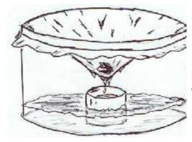
Left: A solar simple still made from a round pan and clear plastic. Place a weighted (so it won't float cup in the center and saltwater in the pan. The sun will distil the water into the cup without the salt.
